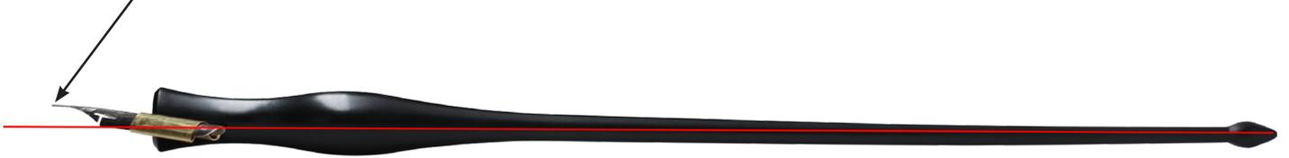
Figure 4: When viewing from the side, the left and the right edges of the nib should align with the center line of the pen holder. In other words, these three points must be in a straight line.
