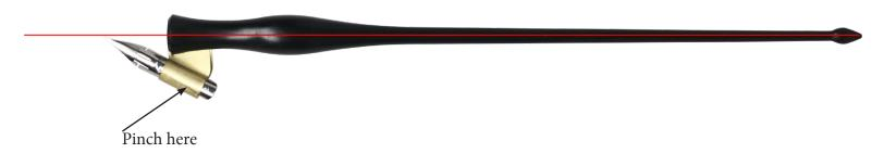
Figure 2: Standard size nibs should be inserted into the metal flange until they are about even with the center of the pen. Some penmen prefer having the nib placed about 2mm or 1/8 of an inch above the center of the pen.
